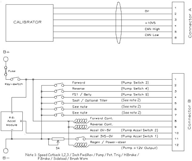
Note 2: Pump Switch 6,7 / Pst. Trig / Pump Inhibit / Motor O.Temp / Brush Worn / Low Oil
