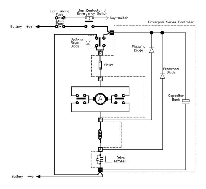
Note: When an emergency battery disconnect switch is fitted, the key switch must be fed through an auxiliary switch to prevent overvoltage damage due to disconnection during regen.
