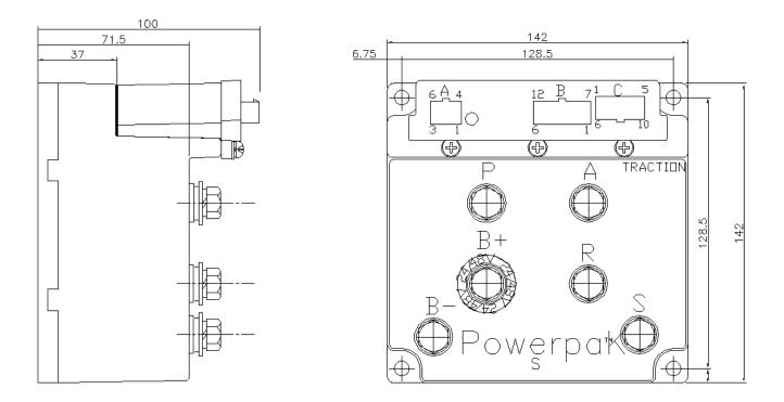
NB: Diagram shows controller with Medium I/O Logic fitted Mounting holes are for M6 bolts.
